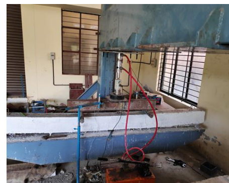
FIGURE 8 TEST SETUP OF BEAM
