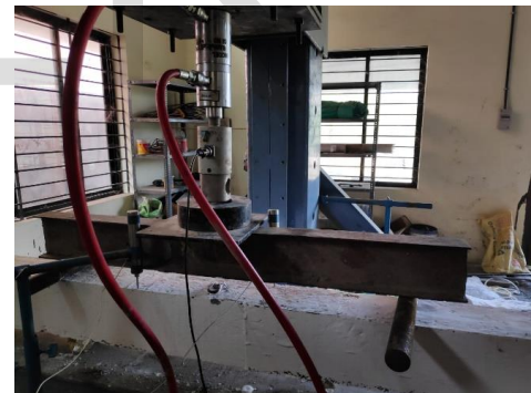
FIGURE 7 TWO POINT LOADING
