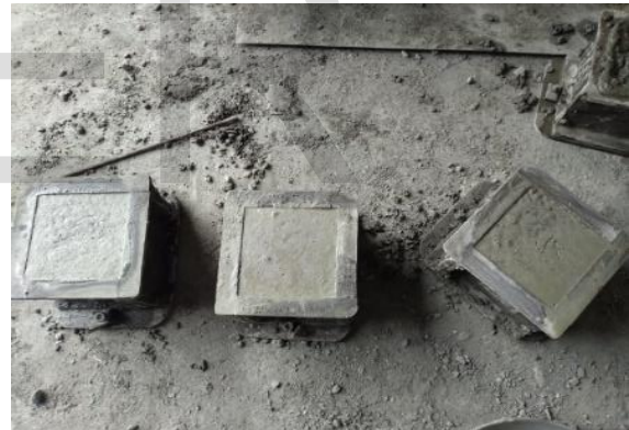
FIGURE 2 CASTING OF CUBES
